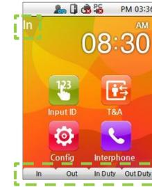
If the T&A mode is set to **Fixed**, the device will automatically log a scheduled T&A event upon authentication. The T&A event cannot be changed. The T&A event schedule can be set using BioStar.
