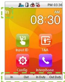
If the T&A mode is set to **Auto**, the device will automatically log a scheduled T&A event upon authentication. The T&A event schedule can be set using BioStar. Different T&A events can still be manually logged using the T&A keys.
