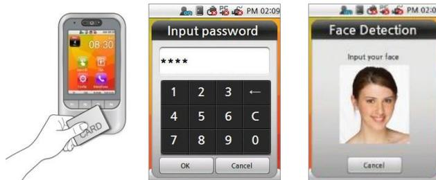
Scan a registered card, enter the corresponding password and then perform face detection.
