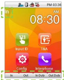
If the T&A mode is set to **Manual Fix**, the device will remain in the last known T&A event. Users can change the T&A event manually by using the T&A keys.
