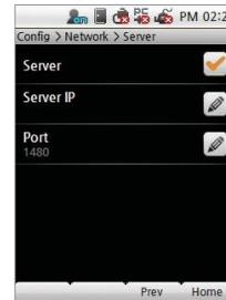
Setup the use of server, IP, and port press **Prev** or **Home** to activate the settings.
