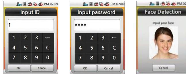
Enter a registered ID, enter the corresponding password and then perform face detection.
