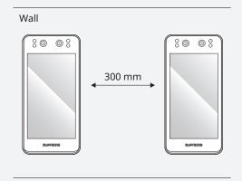
• When using a mobile access card, install devices maintaining a minimum distance of 1 m between devices to avoid BLE interference.
