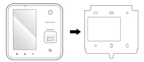
**3** Connect BioStation A2 to the bracket by rotating the product fixing screw of BioStation A2.
